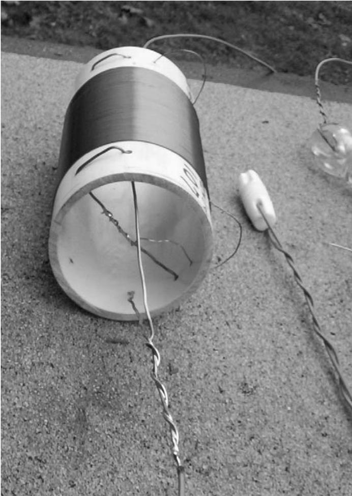
So I had the wires cut, the coils built, and the wires permanently attached to the coils. I left the connections at the center insulator and the end insulators unsoldered, so that I could trim my wire length without having to do it at the coils.
